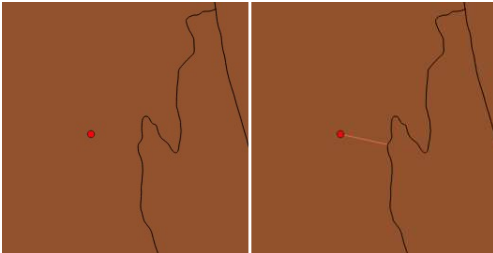
Figure 2: Addition of a new virtual road segment to an existing incomplete road network.
